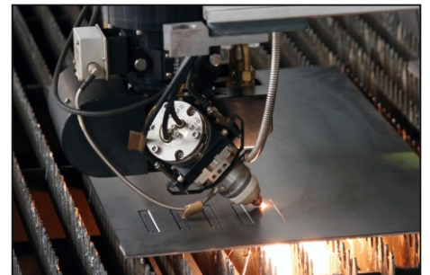
Chamfer laser cutting up to 45° / 16 m
