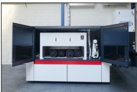
Deburring machine 5,000 x 1,600 mm
