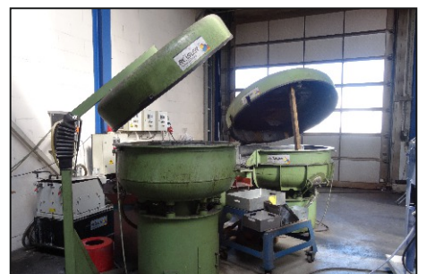
Vibratory grinding machine 100 x 200 mm
