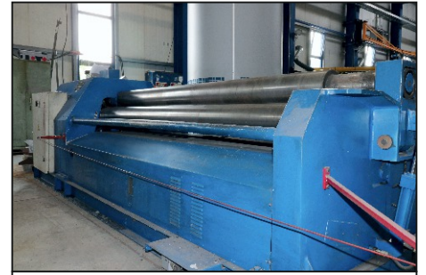
Roll bending machine 2,500 x 6 mm
