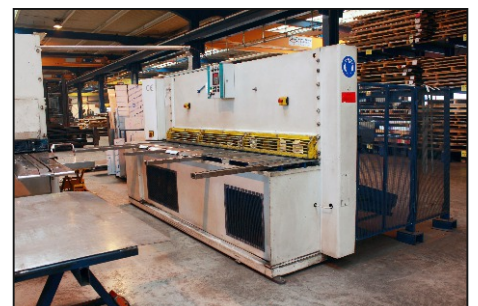
Shearing machine 3,050 x 8 mm
