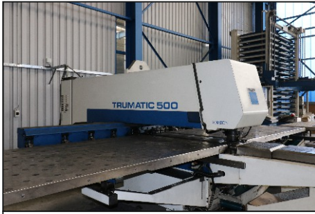
Punching machine 1,600 x 8,000 mm
