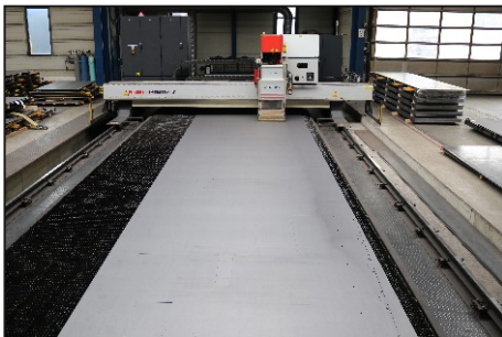
Laser cutting machine 16,000 x 4,000 mm
