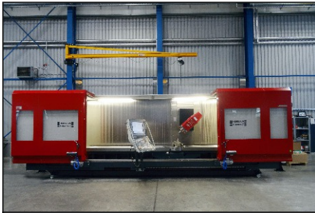
Machining centre 4,200 x 750 x 500 mm
