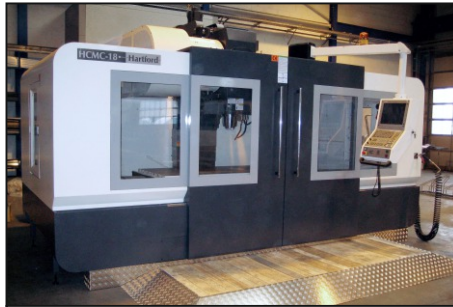
Machining centre 1,800 x 920 x 750 mm
