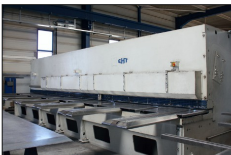
Shearing machine 8,000 x 8 mm
